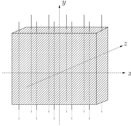
Figure 4: Phantom with a square organization of catheters
