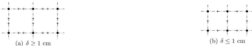
Figure 6: Hyperdose points with a square organization (hyperdose points are represented by a cross, and catheters by a dot)
