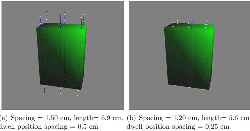
Figure 12: Two different vector dispositions for a parallelepipedic target volume, of width: 3.52 cm, height: 4.90 cm, and depth: 2 cm.
