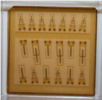
Fig. 3: FEM Langasite plate after the second photolithographic step.
