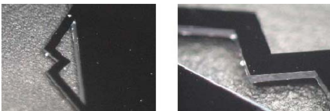
Figure 16: Photography of one of the fabricated W-shaped cantilevers.
