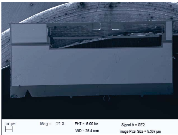
Figure 7. Micro-actuator with electrostatic comb-drives with breaking part, V-groove markers, and flexure springs for assembly (design B).
