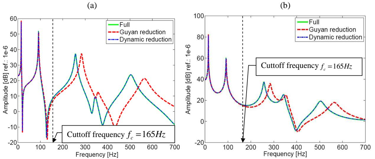
**Fig.7.** FRFs for full and reduced models: Dynamic/Guyan reduction methods: (a) Point P- (b) Point K of the viscoelastic sandwich beam
