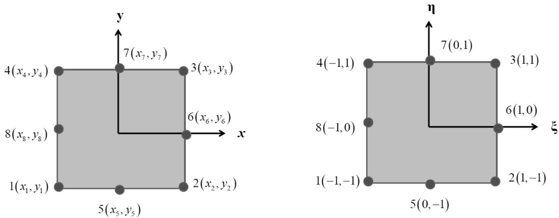
**Fig.2.** Serendip finite element in: (A) elementary coordinates, (B) local coordinates
