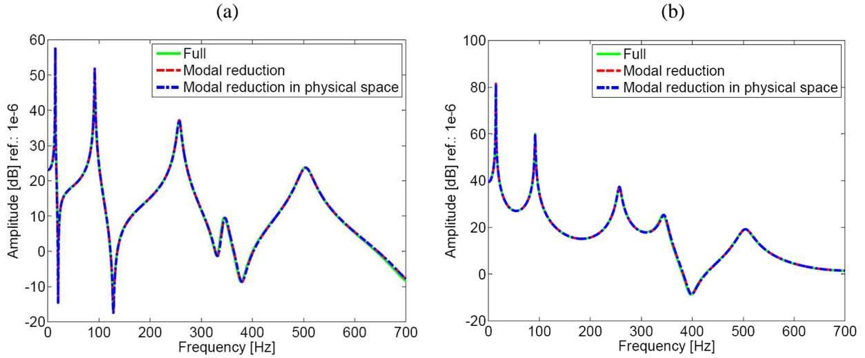
**Fig.8.** FRFs for full and reduced models: Modal/Modal in physical space reduction methods:
