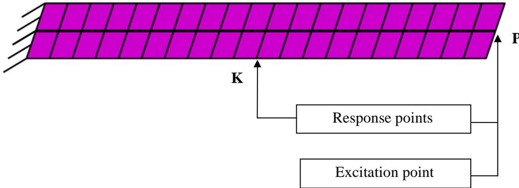
**Fig.3.** Clamped-Free(C-F) sandwich beam finite element
