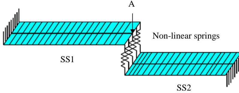
**Fig.19.** FE model of the global non-linear assembled viscoelastic sandwich beam
