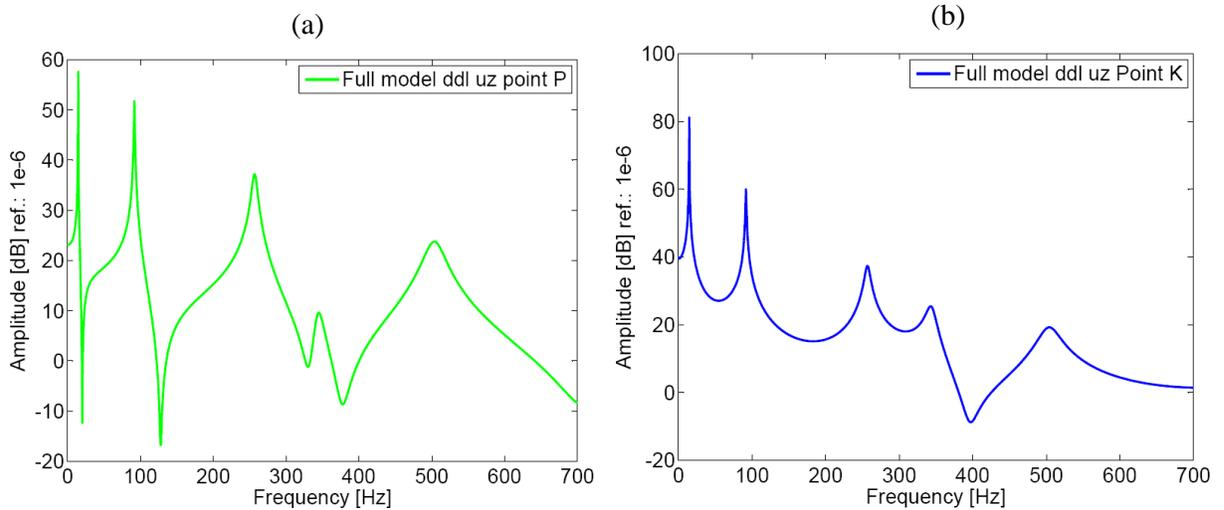
**Fig.4.** FRFs of the full GHM model plotted in: (a) Point P- (b) Point K
