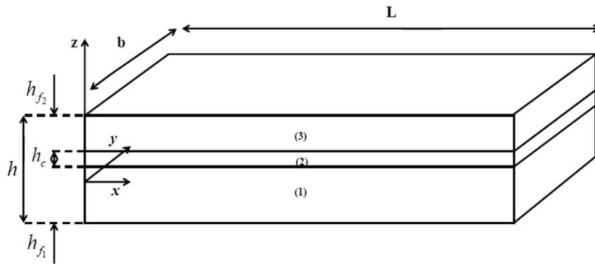
**Fig.1.** Sandwich structure geometry
