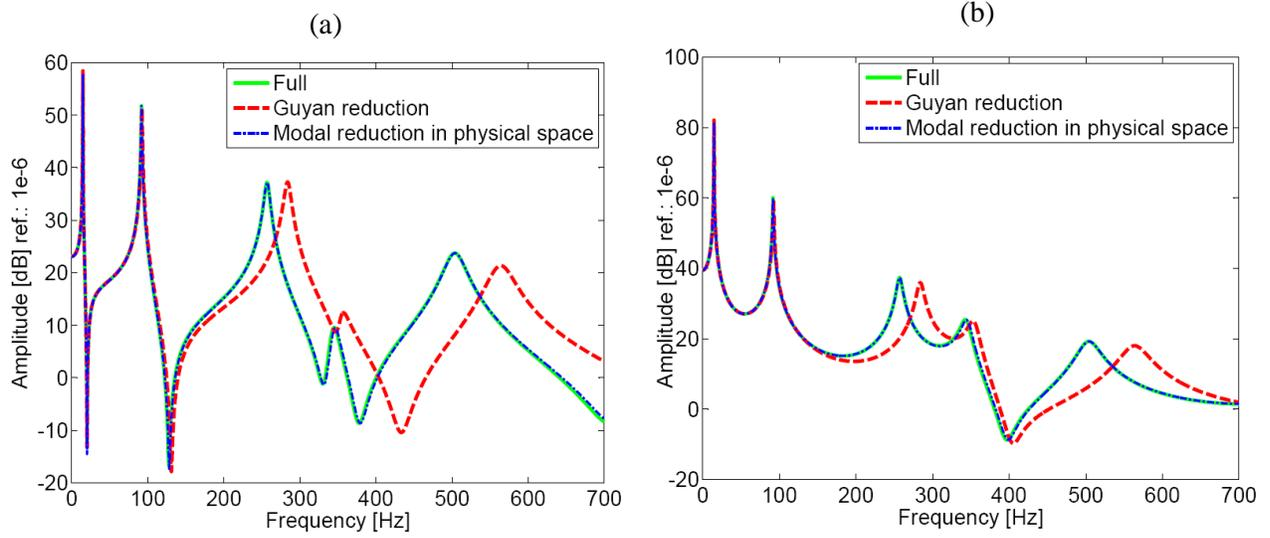
**Fig.9.** FRFs for full and reduced models: Guyan/Modal in physical space reduction methods:
