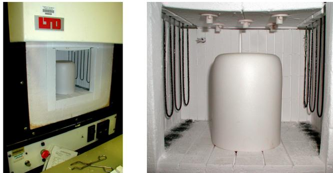
Fig. 1: Lenton chamber furnace for sapphire annealing
