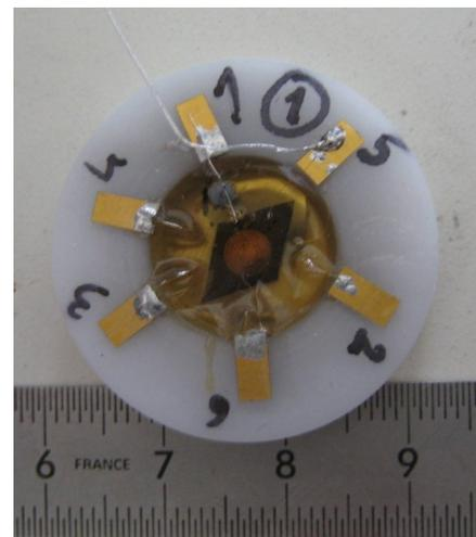
Figure 4: Photo of the whole probe after backing filling and electrical connection for characterization tests (the back side is grounded)
